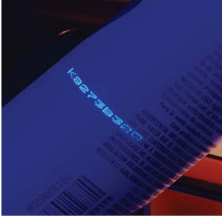
For customers requiring a discreet and covert coding option, there is SigNature molecular-tagged ink **V4259M** (commercially known as V4259). Intended as a complement to V4221M and applicable to the same wide range of substrates, this ink is clear and fluoresces blue under ultraviolet light. V4221M and V4259M can be used together on one item, for customers requiring an invisible security option to track and secure their products beyond traditional overt product marking.
