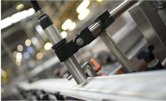
Established in the 1970s, continuous inkjet printing (CIJ) is still the coding option of choice among many industries today, and for good reasons. CIJ coding is an affordable, high-volume solution, compatible with multiple substrates, fast-drying, durable, and meets identification requirements across a wide range of products and packaging. The aim of every manufacturer is to keep production lines moving, without sacrificing quality compliance in the proper
