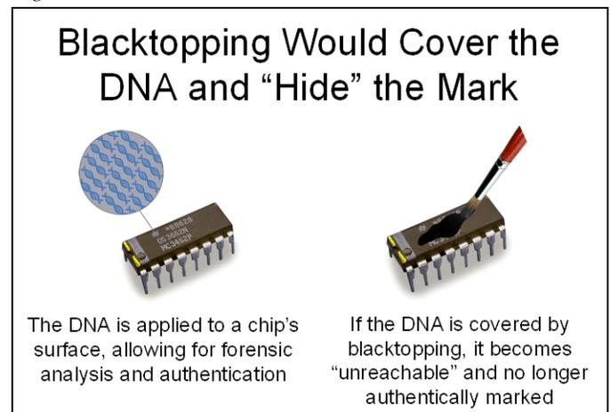
**Reused DNA Blacktop** (Figure 3) Cannot be authenticated. Loss of structure during transfer disables the mark. It will not pass its authentication program.
