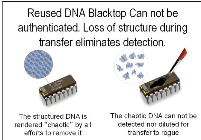
**Repackaging** DNA is obscured even by partial repackaging. If repackaged, the DNA mark will not be detected, thus the chip will not pass an authentication program.
