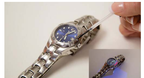
Quick Trace in the Field - under UV light, the DNAet mark emits a bright red signal, making it easy to identify on the spot.
